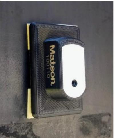
Accelerometer, temperature, gyroscope, humidity, magnetometer, pressure sensors
